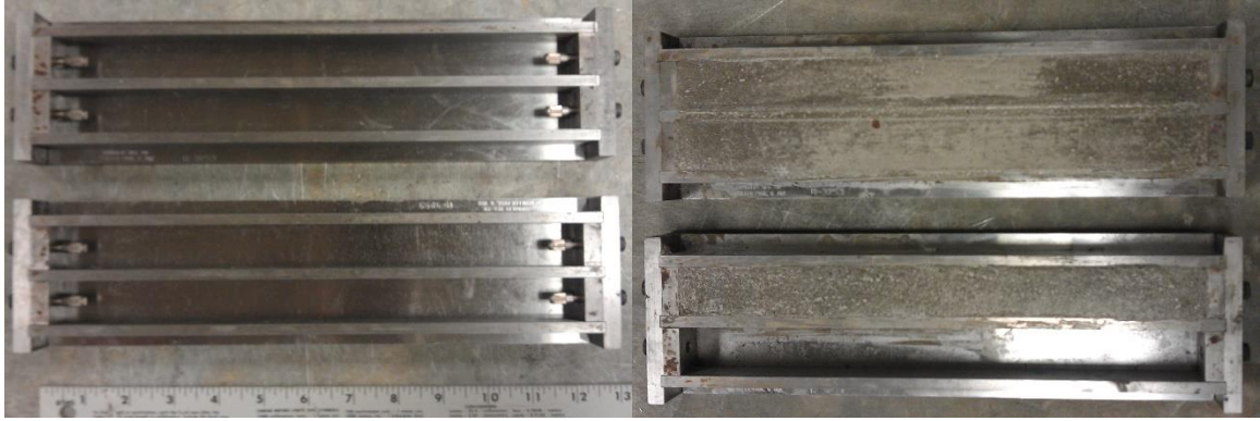
Figure 2.4. Mortar-Bar mold with gage studs (left) and mortar-bar mold with three mortar-bars (right). Picture used with permission from Richard Deschenes.
