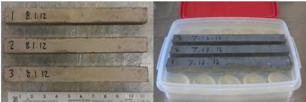
Figure 2.5. Mortar-bars (left) and mortar-bar in storage container (right). Picture used with permission from Richard Deschenes.
